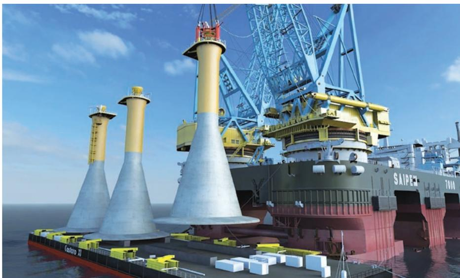
➤ **Bouygues Travaux Publics (mandatory, 40.5%) in consortium with Saipem (40.5%) and Boskalis (19%) have been awarded the design work, construction and installation scope for 71 concrete Gravity-Based Structures (GBS) as foundation for the Fécamp offshore wind farm in Normandy, France. The award was made by EDF Renewables, Enbridge Inc. and wpd Offshore. The contract carries a total value of 552 million euros.**
