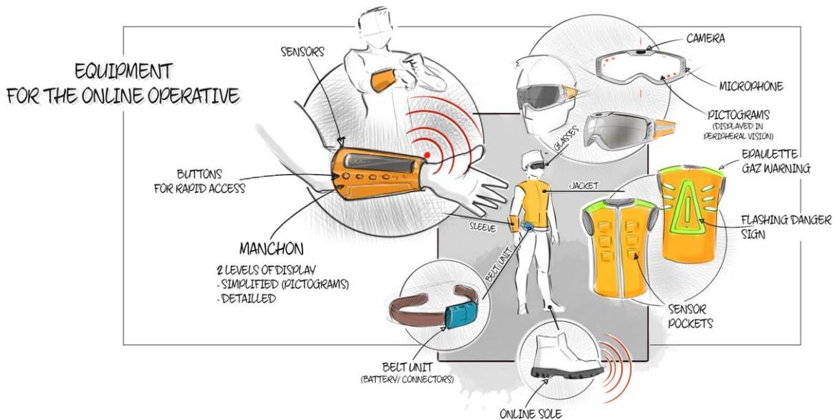
**A modular range of equipment allowing communication, analysis of the environment and transmission of relevant production information.**
